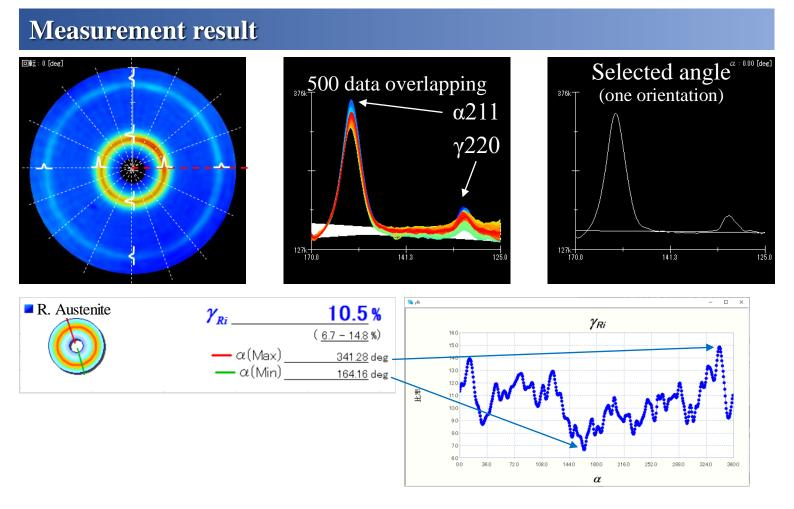
Results of 500 orientation can output at one measurement!
