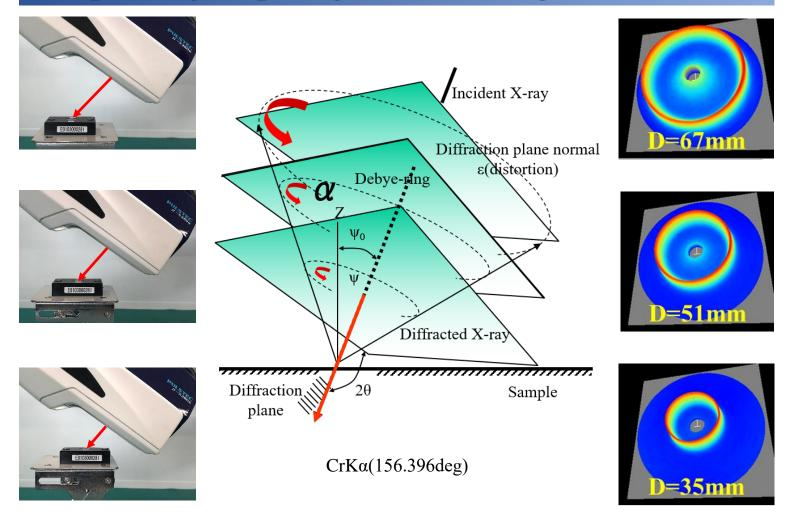
As Debye-ring's size is changed according to the sample distance, measurement is possible if the Debye-ring is within the 2D detector.
