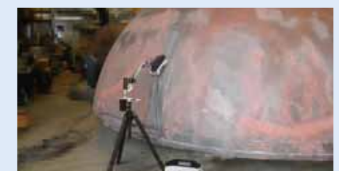
Storage tanks : Weld and annealing effects
